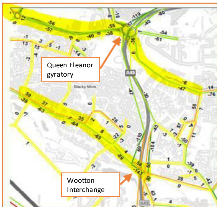
Figure 2: 2031 evening peak hour flow reassignment (D1 vs J1c)
